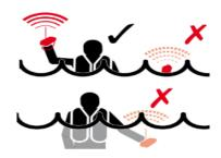
✓ Ensure that the area marked "GPS Zone" is not obstructed or covered in any way and always has a clear view of the sky.
